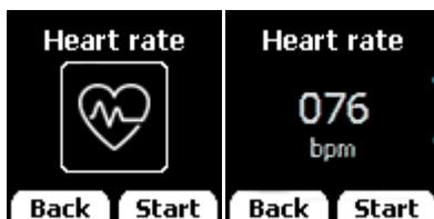
Heart-rate readings from the optical sensor. Two wavelengths of light from two LEDs (red and green) are emitted from the small slit on the rear of Hexiwear. When you place your wrist or fingertip over the slit, the sensor measures the light absorbance of pulsing blood through a photodetector and derives heart-rate info. Current firmware version is able to show rough estimates.
