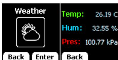
Shows ambient temperature, humidity and pressure data in real time.
