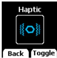
Toggles haptic feedback engine on and off. White when turned OFF, Blue when turned ON. Haptic engine gives tactile feedback on button presses. Deactivating it conserves battery.
