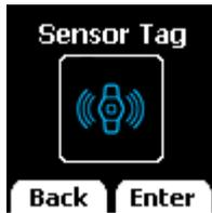
Toggles Sensor tag mode. When active, Hexiwear will continually broadcast readings from all its internal sensors over BLE. The readings can be accessed from the Hexiwear smartphone app, or directly from the WolkSense cloud. White when turned OFF, Blue when turned ON.
