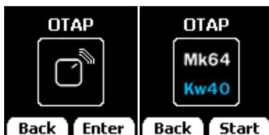
OTAP stands for "Over the Air Programming e.g. wireless firmware updating. You can choose to update either the KW64 (main MCU) or the KW40 (BLE chip). Requires Hexiwear smartphone app. [See this video for instructions.](#)
