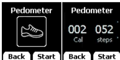
Step and calorie counter next to each other. Walking steps are inferred from accelerometer readings. Calories are calculated using a formula. "Stop" button resets count.
