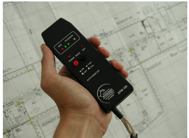
Figure 12: EPM 100 helps to qualify installation positions
