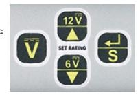
ENTER: Press to select the reference value, to start the test, and to display conductance in siemens (S)
