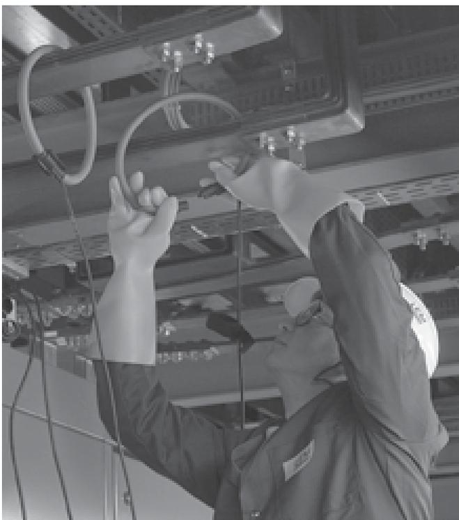
Fig. 40 Typical LEM-flex use, surrounding conductor(s) and latched.
