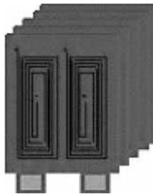
Figure 43: PRiME™ sensor multi-layers printed wiring board
