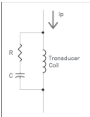
Figure 6: Schematic of high frequency bypass
