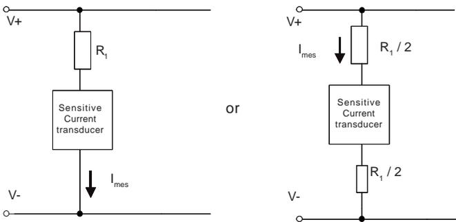
Figure 21: A basic principle for voltage measurement
