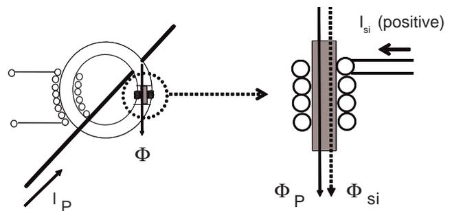
Figure 25: Standard Fluxgate - gap flux distribution – additive flux
