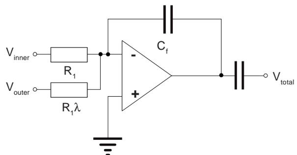
Figure 45: PRiME™ – processing of the coil signals
