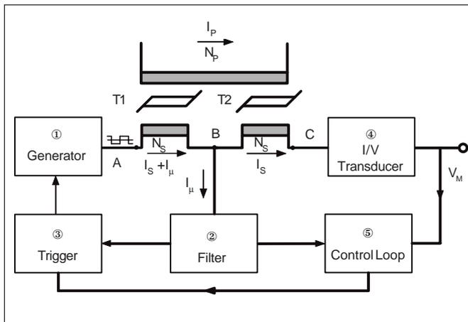
Figure 34: Block diagram of the C-type Fluxgate transducers
