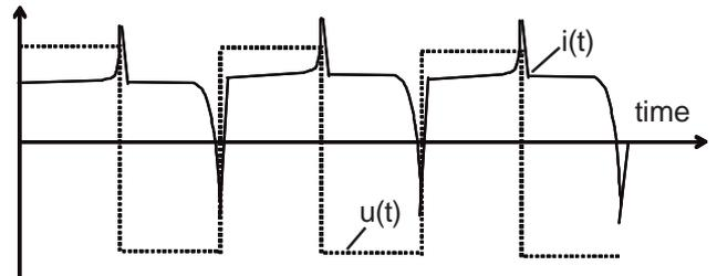
Figure 32: Voltage steps and current response ( $I_p \neq 0$ )
