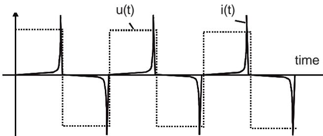
Figure 31: Voltage steps and current response ( $I_p = 0$ )
