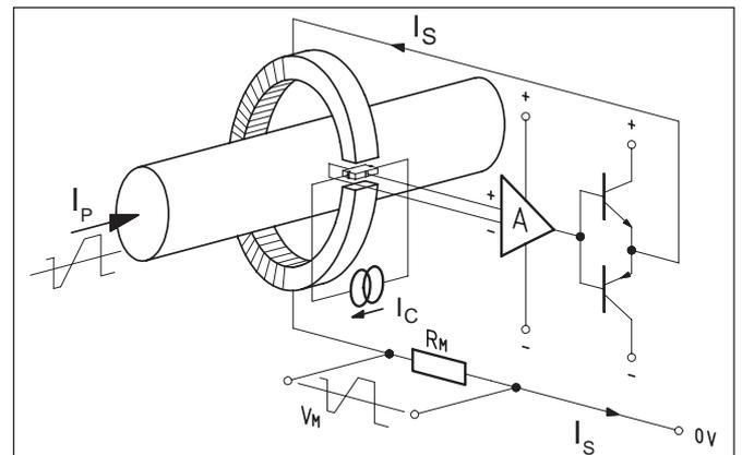
Figure 10: Operating principle of the closed loop transducer
