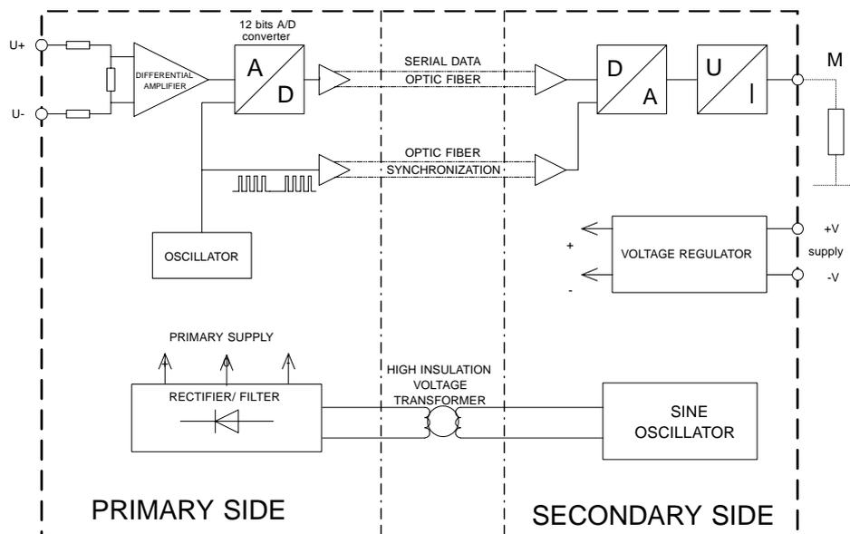
Figure 47: OptiLEM working principle
