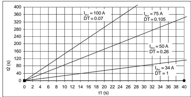
Fig. 16 Overload diagram of the LTS 25-NP for a rest current of 25 A<sub>rms</sub>, linear zone
