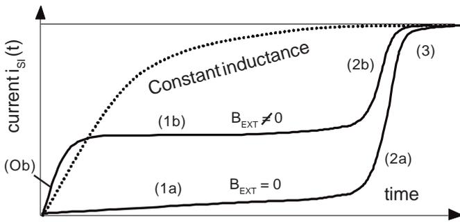
Figure 30: Current response to a voltage step – Fluxgate sensing head ( $B_{EXT}$  set at a parameter)
