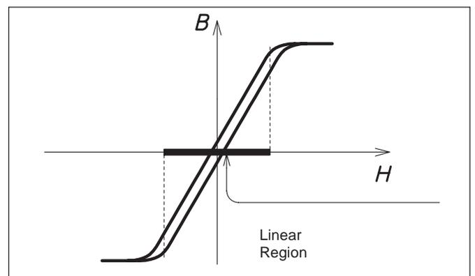
Figure 4: Magnetization curve
