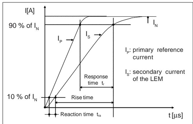
Figure 8: Definition of the transient response parameters
