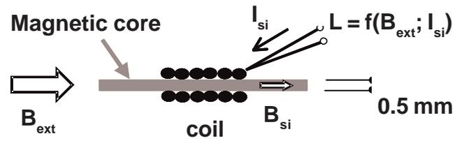
Figure 24: Fluxgate magnetic sensing head (saturable inductor)
