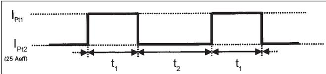
Figure 14: Periodic overload with a standby current of 25 A at 85 °C
