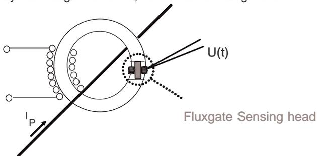
Figure 23: Structure of the „standard Fluxgate“
