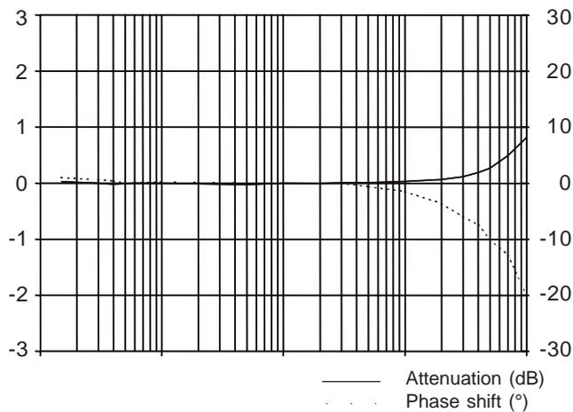
Figure 46: PRIME™ – typical bandwidth 5 to 100 kHz
