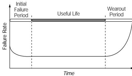
Life Cycle of an Aluminum Electrolytic Capacitor
